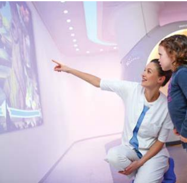
With the Philips Ambient Experience patient in-bore solution for MR, engaging visuals are displayed on the back wall and can be seen via a mirror on the head coil, while patients can listen to music/sound through the headphone.
